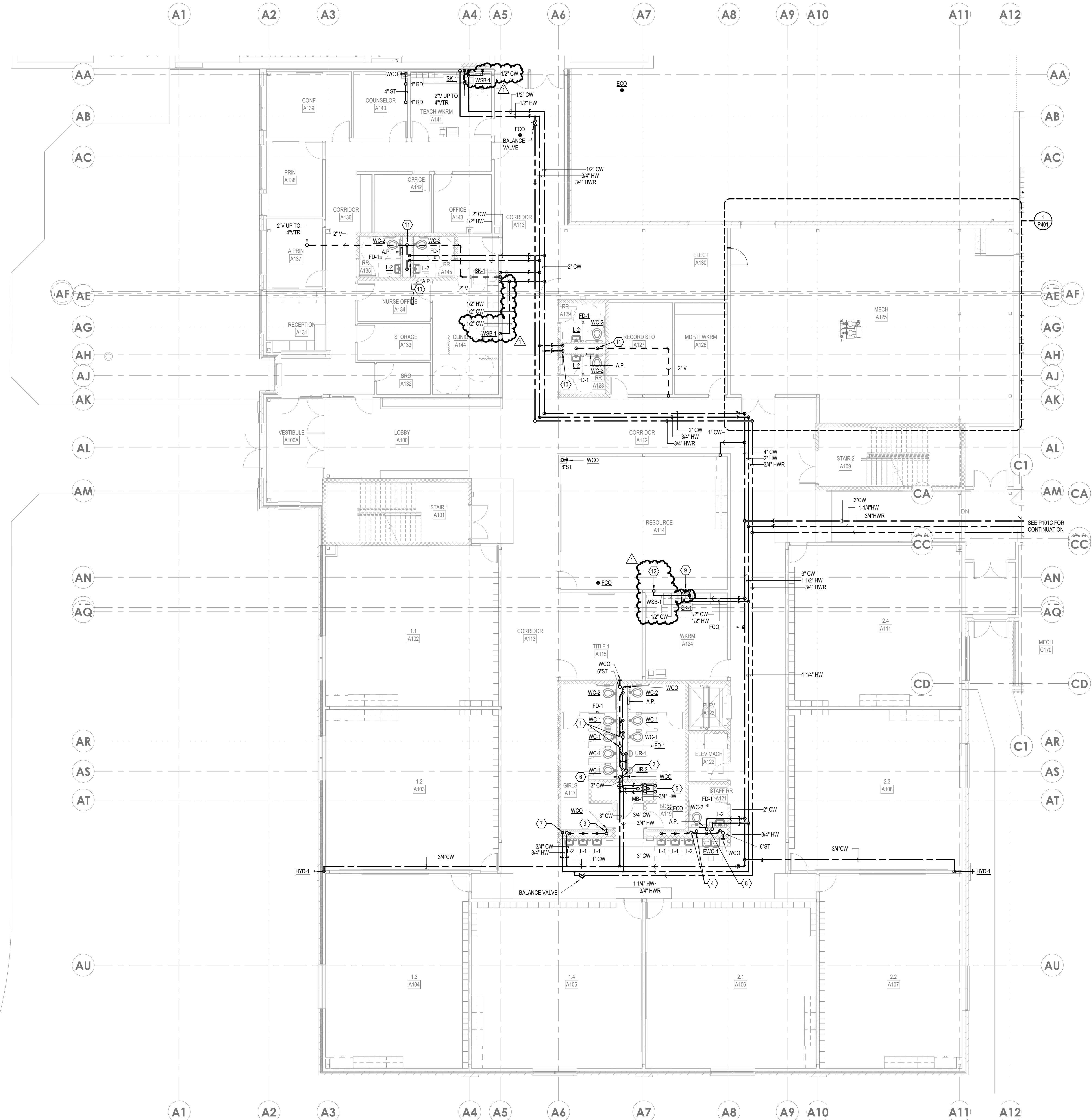
1 FIRST FLOOR PLUMBING PLAN - UNIT A 1/8" = 1'-0"
