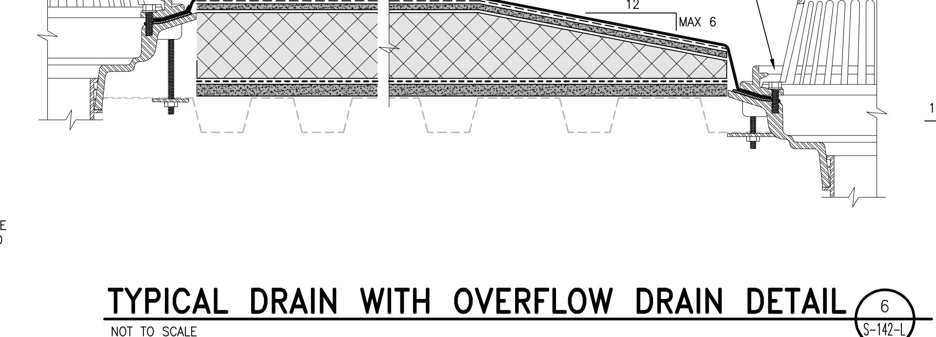
TYPICAL DRAIN WITH OVERFLOW DRAIN DETAIL
