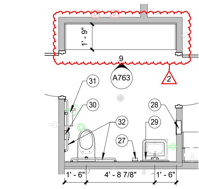
**4** ENLARGED FLOOR PLAN - RESTROOM A1a
