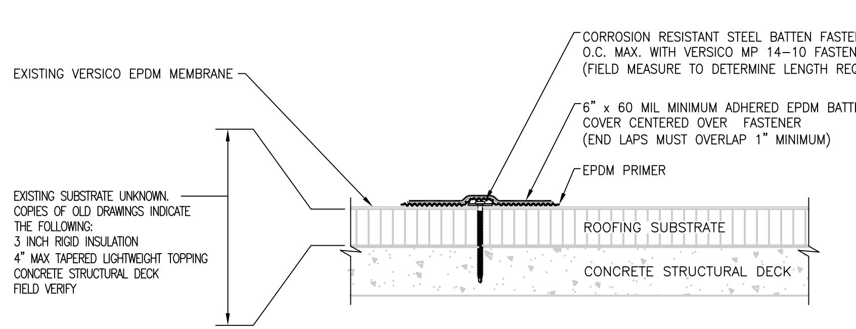
TYPICAL BATTEN SEAM REPAIR DETAIL
