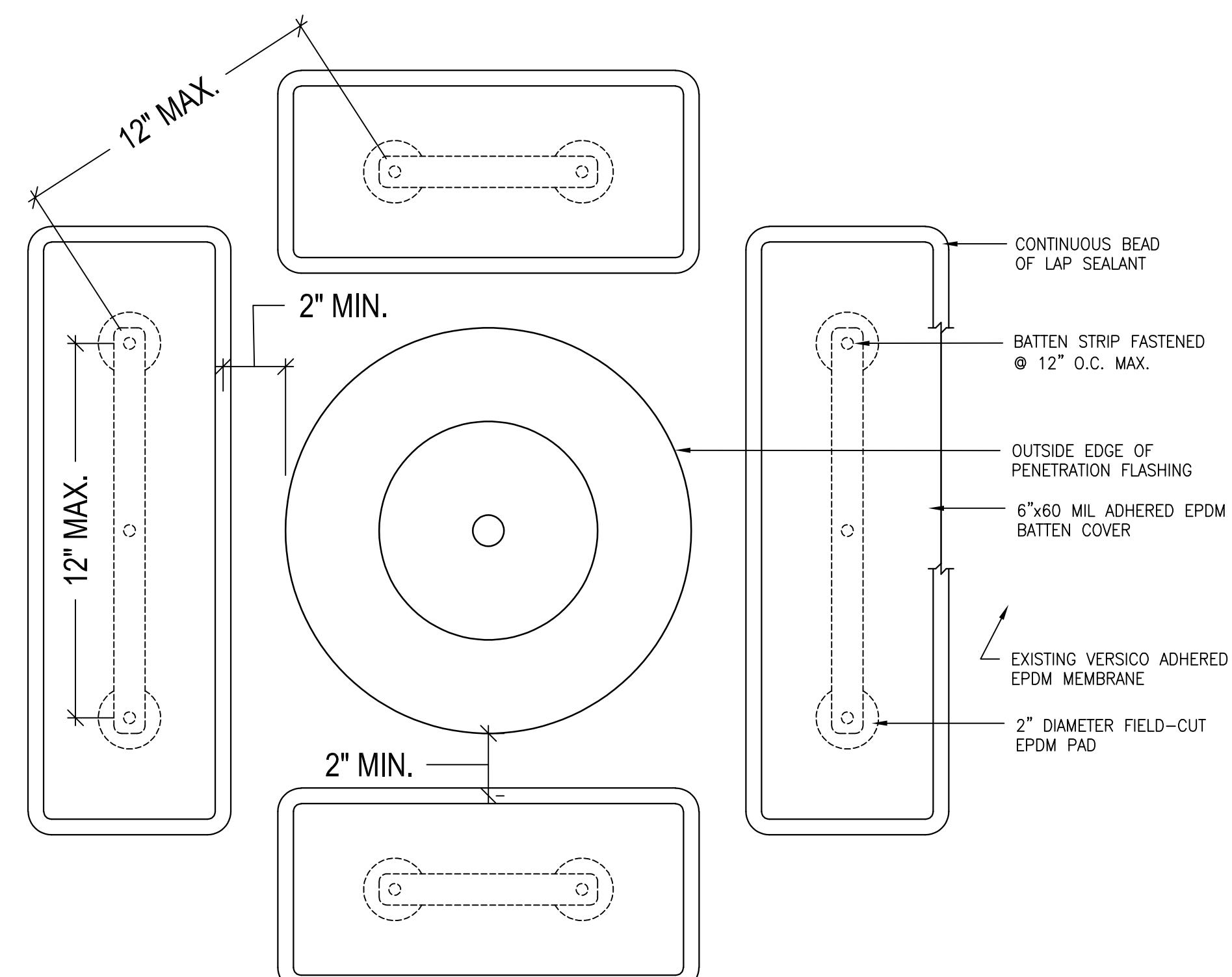
TYPICAL BATTEN DETAIL @ ROOF PENETRATION
