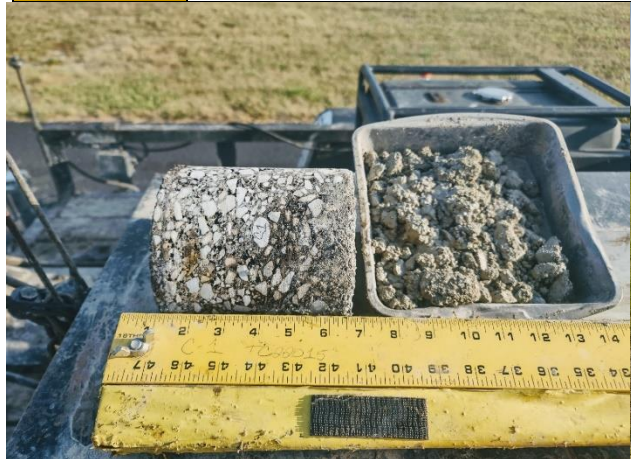
Figure 1a: C-1 Core Photograph
