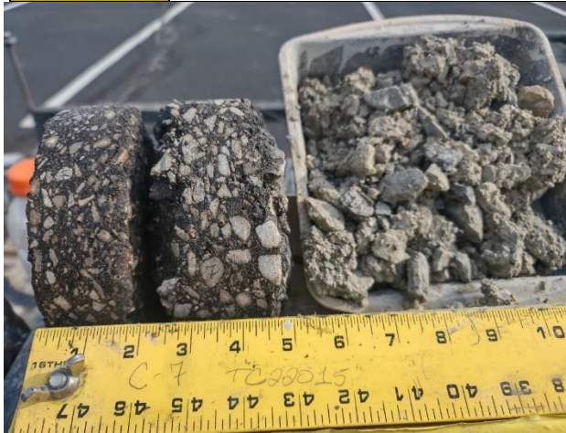
Figure 7a: C-7 Core Photograph
