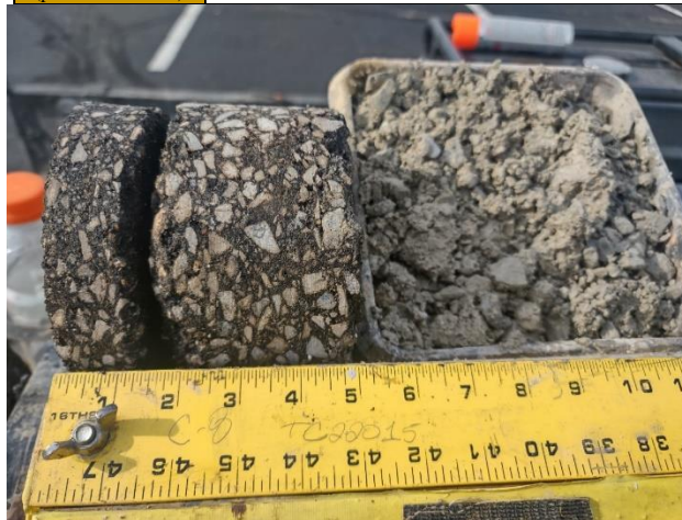
Figure 8a: C-8 Core Photograph
