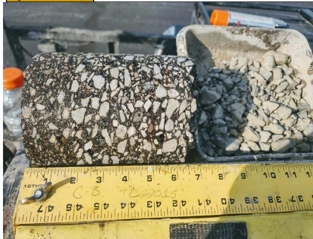
Figure 3a: C-3 Core Photograph
