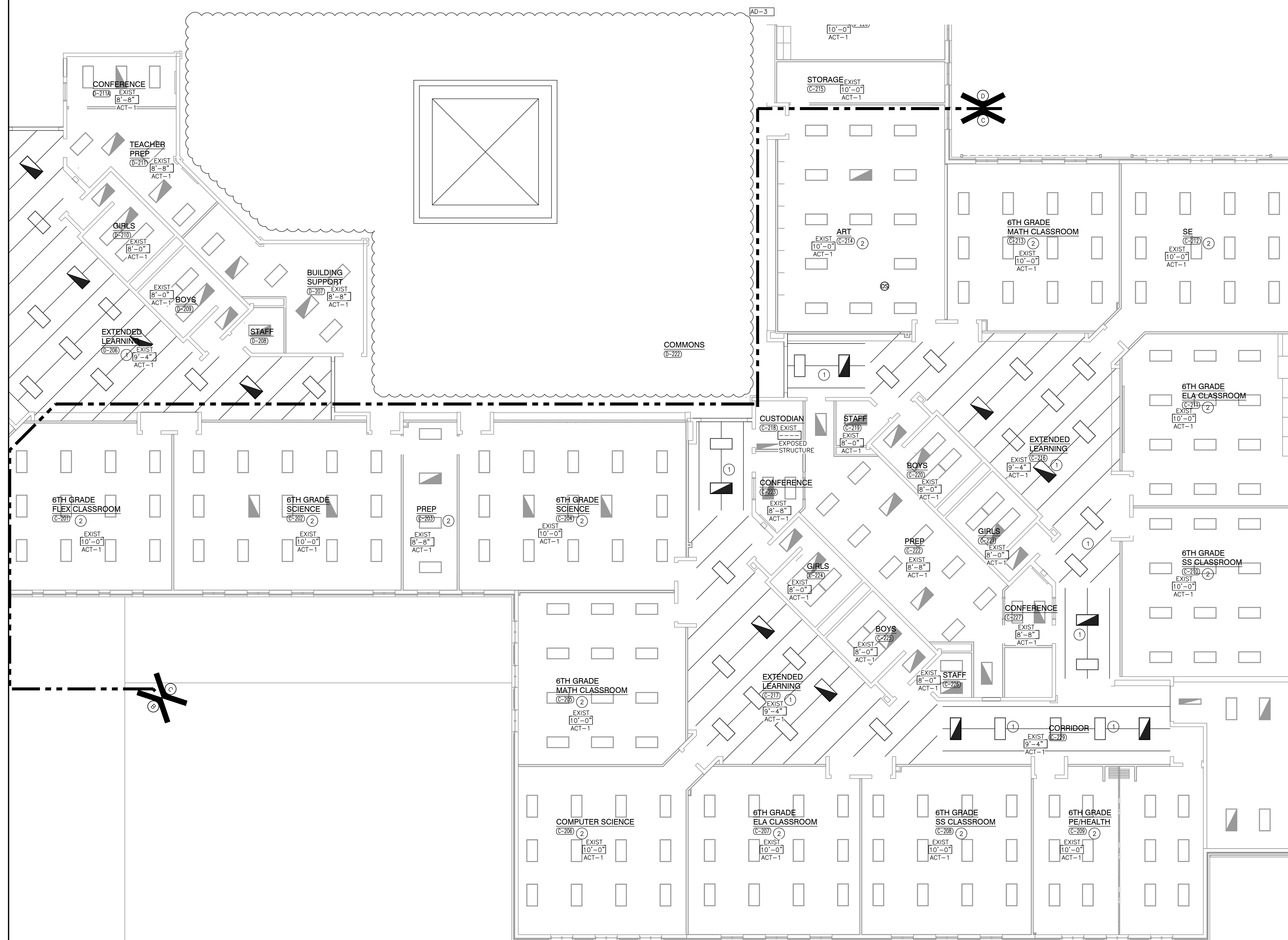
UNIT "C" ARCHITECTURAL SECOND FLOOR REFLECTED CEILING PLAN
