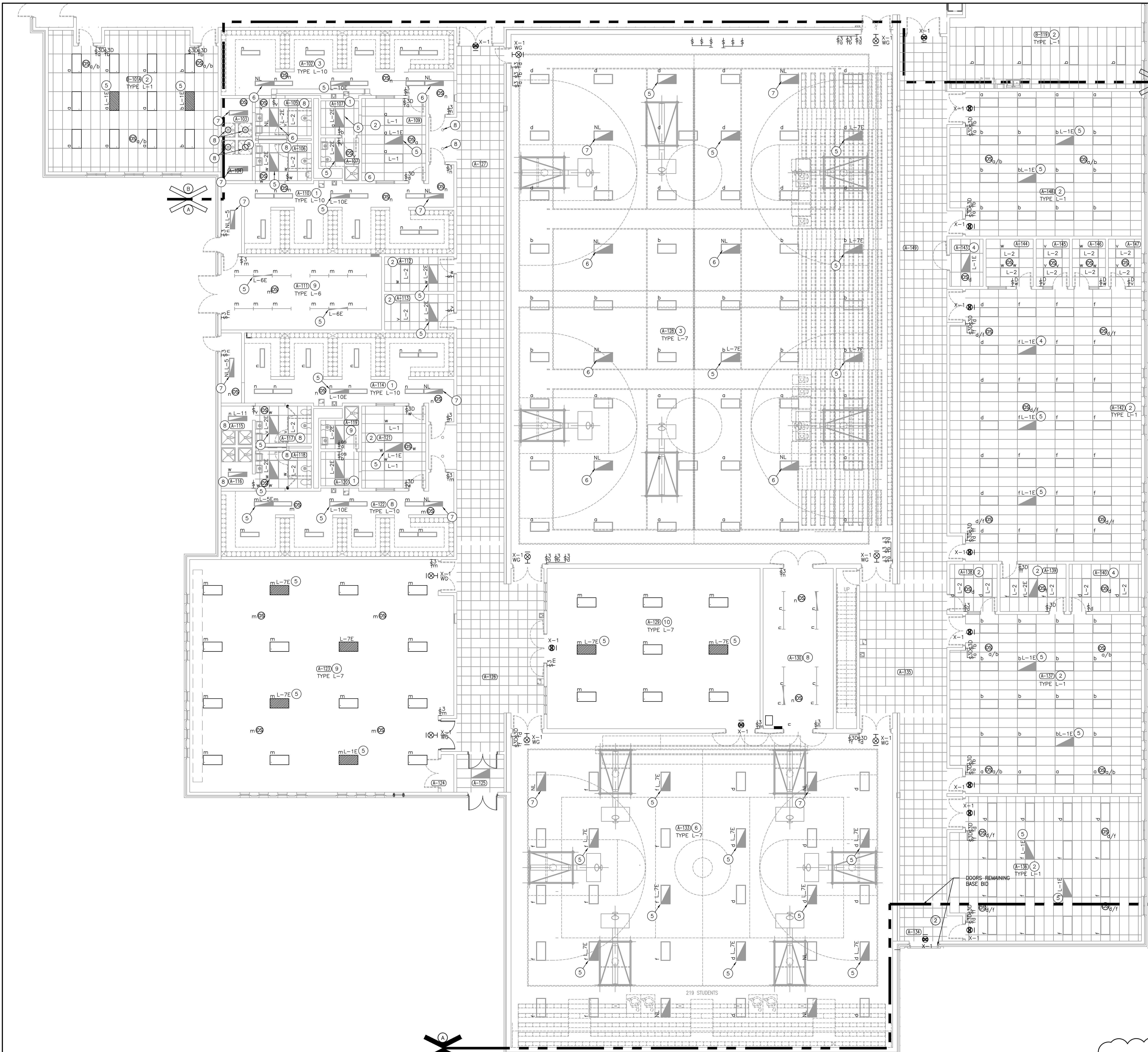
UNIT "A" ELECTRICAL FIRST FLOOR LIGHTING PLAN - ALTERNATE BID
