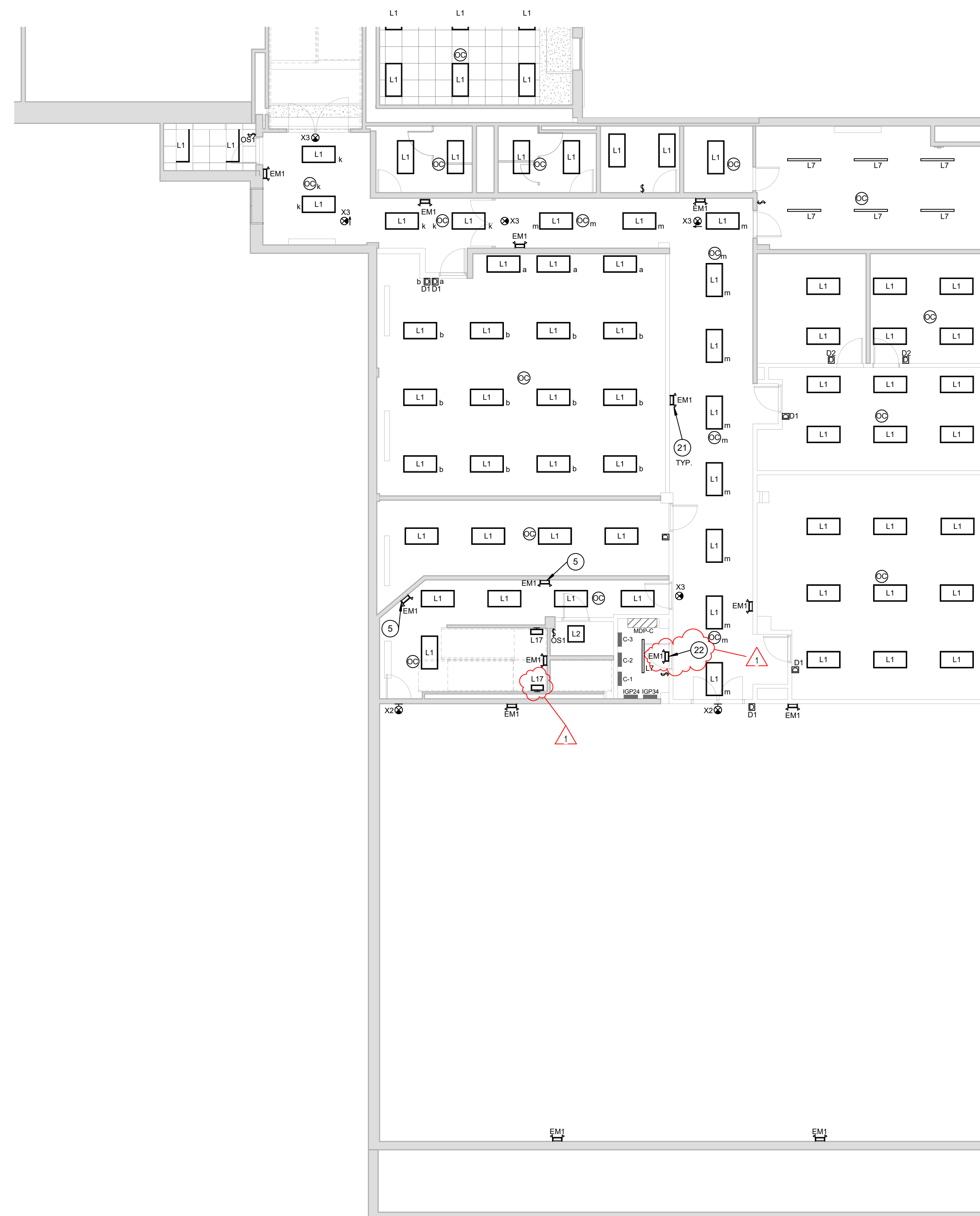
1 SECOND FLOOR ELECTRICAL PLAN - UNIT C 1/8" = 1'-0"
