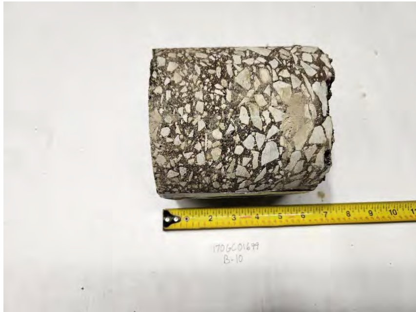
Figure B-10.3 Recovered Pavement Core
