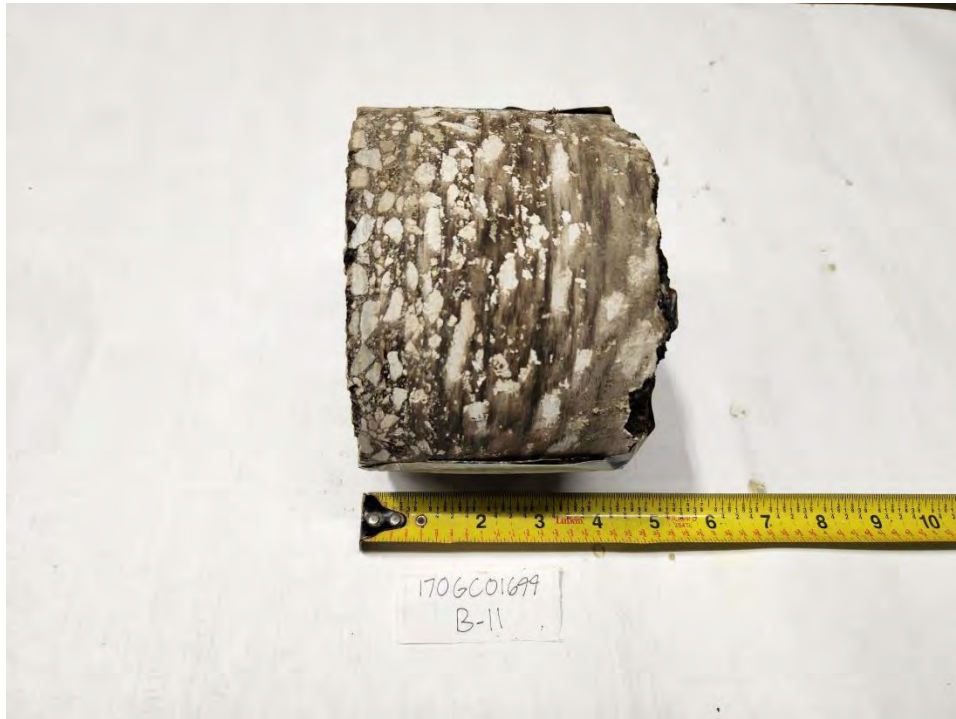
Figure B-11.3 Recovered Pavement Core
