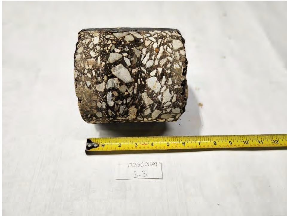
Figure B-3.3 Recovered Pavement Core
