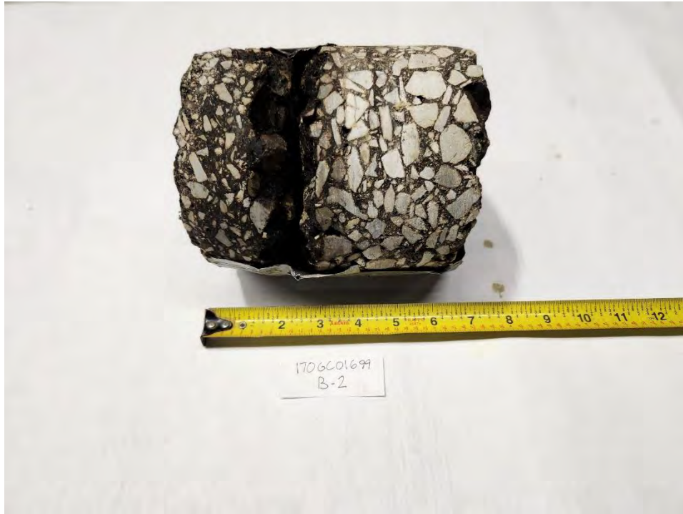
Figure B-2.3 Recovered Pavement Core
