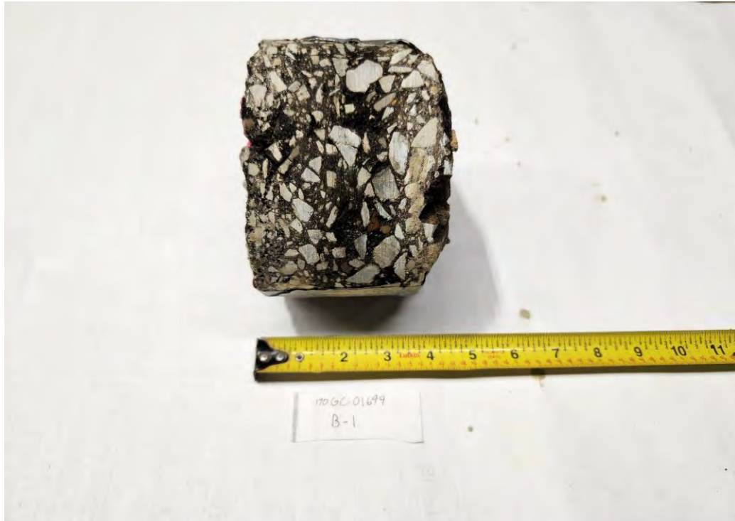
Figure B-1.3 Recovered Pavement Core
