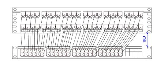
SWITCH - PATCH PANEL CROSS CONNECT SAMPLE
