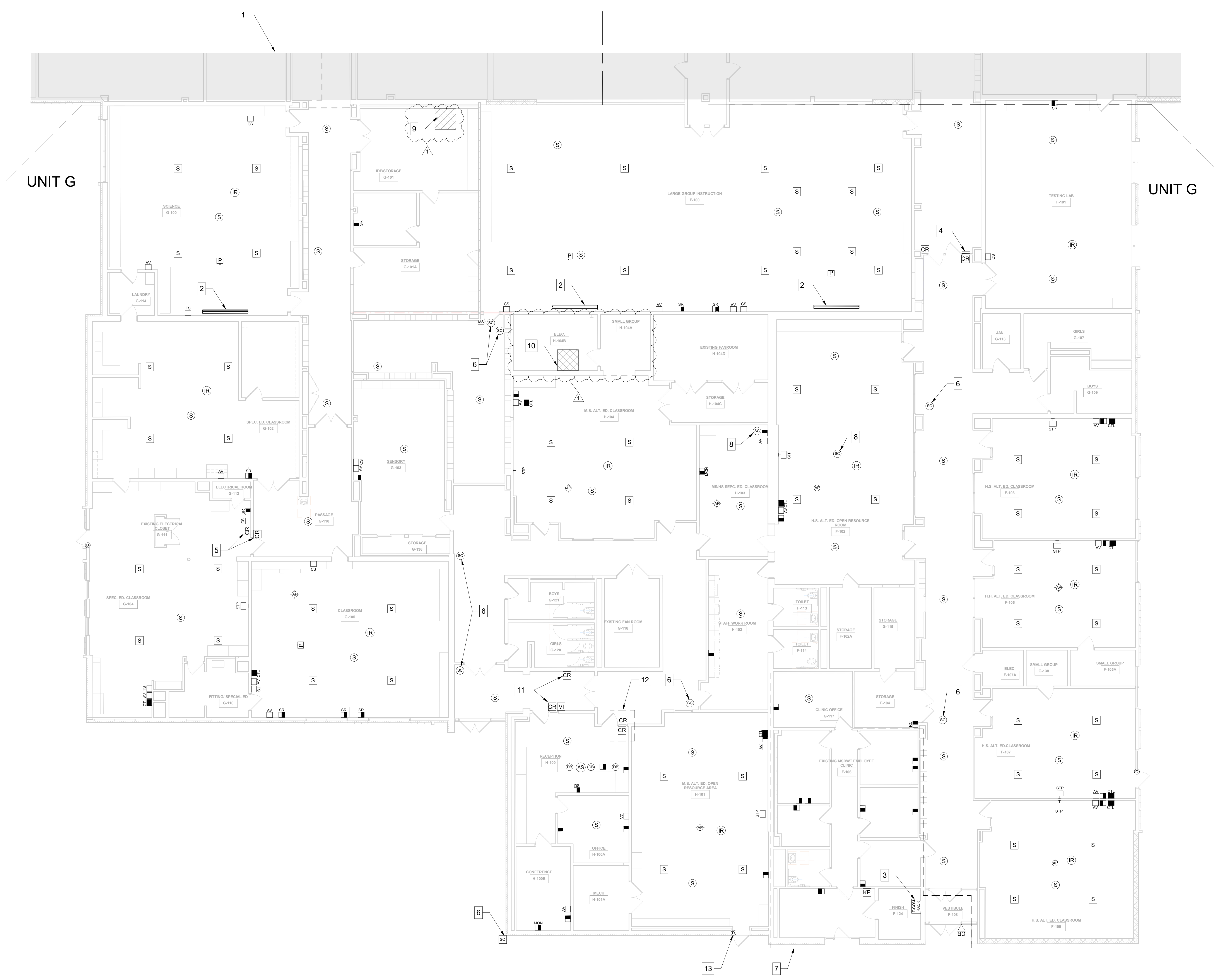
FIRST FLOOR DEMOLITION PLAN 1 - UNIT G 1/8" = 1'-0"
