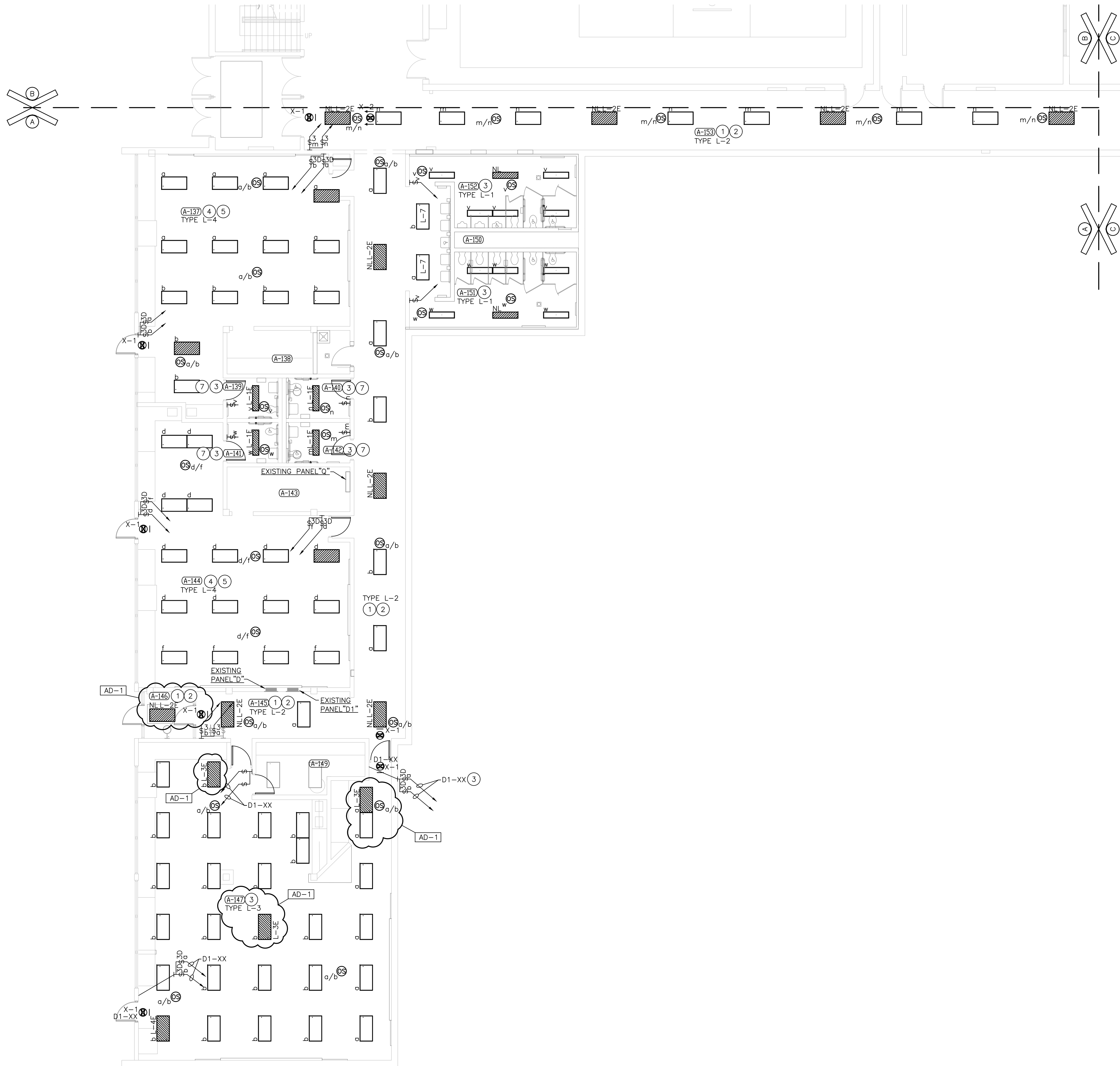
UNIT "A" LOWER LEVEL ELECTRICAL LIGHTING PLAN SCALE: 1/8" = 1'-0"
