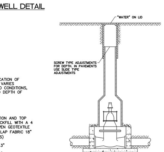
**TYPICAL VALVE BOX INSTALLATION**
