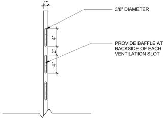
9 ACM PANEL VENTILATION SLOT DETAIL
