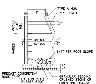
**SANITARY MANHOLE (IEPA TYPES A AND C)**
