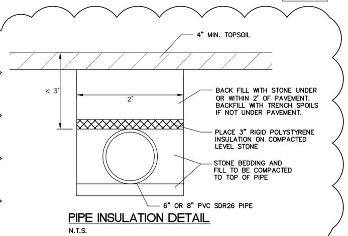
**PIPE INSULATION DETAIL**
