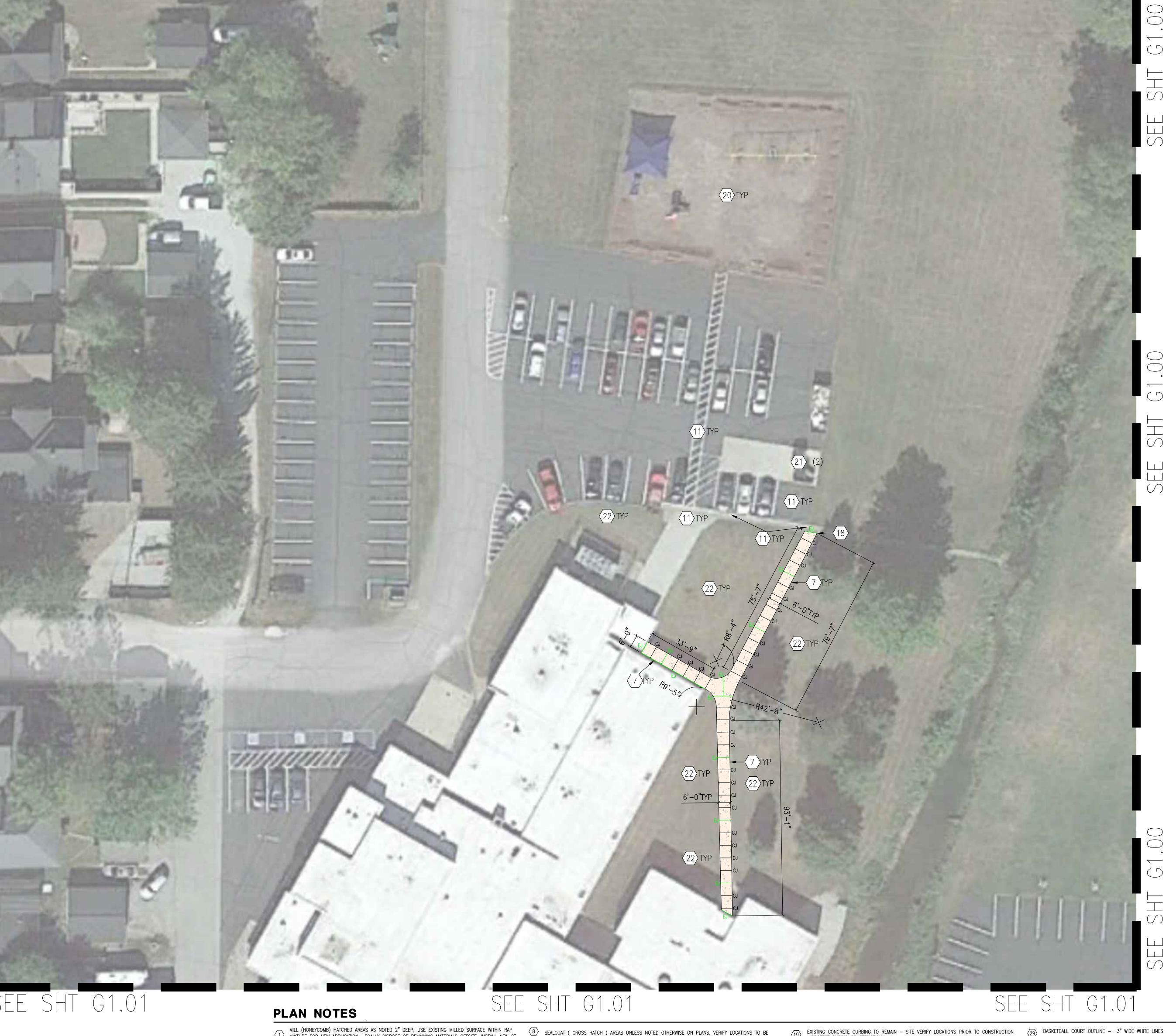
$\frac{1}{2}$  MIXTURE FOR NEW APPLICATION, LEGALLY DISPOSE OF REMAINING MATERIALS OFFSITE. INSTALL NEW 2" RECYCLED ASPHALT PAVEMENT (RAP) SURFACE COURSE PER DETAIL #1 SHT G4.0. PROVIDE POSITIVE DRAINAGE TO EXISTING STORM INLETS TYP. AREAS SHOWN ARE APPRÖXIMATE AND SHALL BE FIELD
