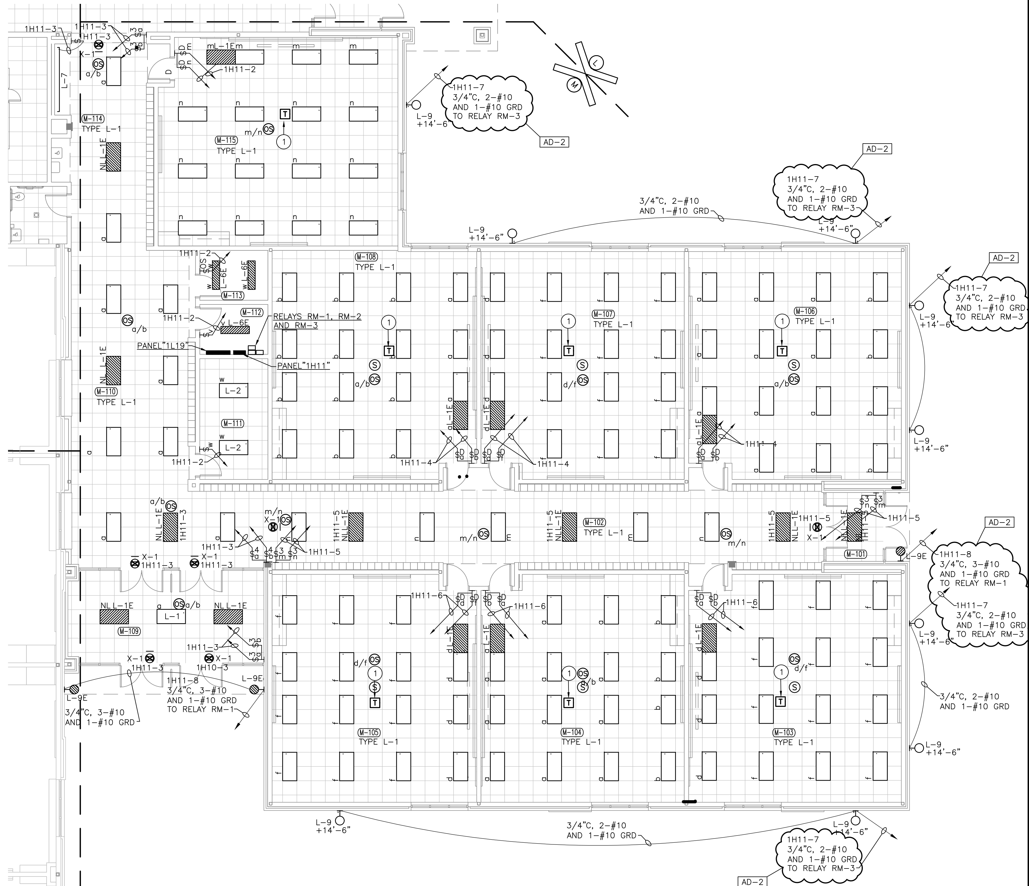
UNIT "M" ELECTRICAL FIRST FLOOR LIGHTING PLAN
