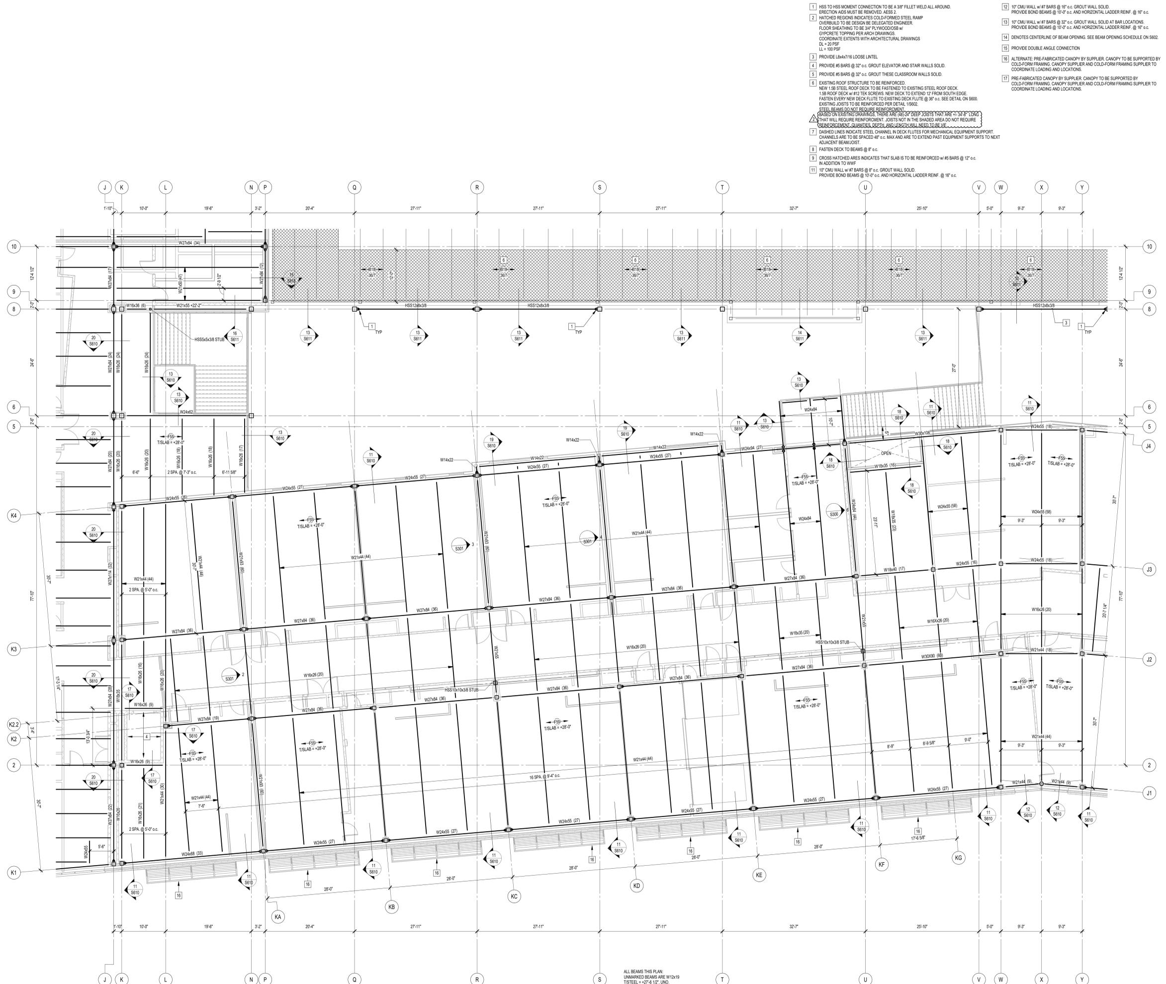
ALL BEAMS THIS PLAN UNMARKED BEAMS ARE W12x19 T/STEEL = 27.5 1/2" UNO.
